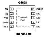
Note: Recommend connecting the Thermal Pad to the GND or let it keep floating.
